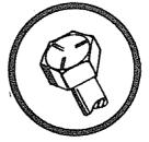
A GRADE 5 HEAT TREATED BOLT CAN BE IDENTIFIED BY THREE LINES INDICATED ON THE BOLT HEAD AS SHOWN AT LEFT.
